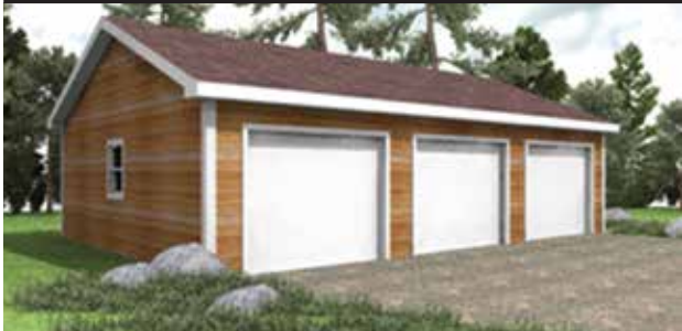
Yukon: 24' x 36' 3-Bay • 2 x 4 x 8 Framing 24" on - center • 7/16" OSB wall sheathing • 5/8" roof sheathing • 25 Year three tab shingles • 4 - Single hung vinyl windows • 1- 3'0" x 6'8" Premium steel door • 3- 9' x 7' Steel, non-insulated classic raised panel garage doors
